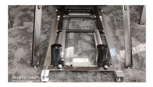
There should be approximately 6 inches from the front pinball legs to the front of the EZ Lift device frame. This distance will be greater if used on shorter machine cabinets such as Gotliebs. A safety strap will be installed in this location at a later step.
